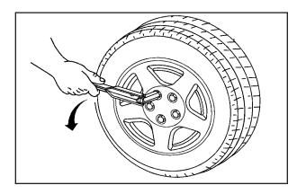
4. Use the wheel wrench to loosen all the wheel nuts. Do not remove them yet.
